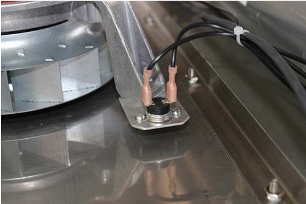
Top Oven Compartment Thermostat set to 145°F
